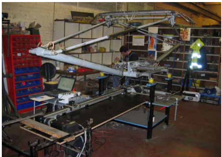
Figure 11: Pantograph with DTK's contact force measuring equipment
